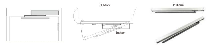
Push Arm Installation: Suitable for door wing opening outward (drive system inside)
